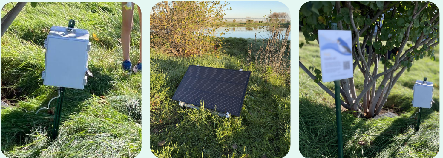
Figure 4. The PAM device is housed in an electrical box, mounted on a garden stake (left), and connected either to an outdoor outlet or to a solar panel system (middle). We highly recommend including a sign (right) to alert passersby that a listening device is present.
