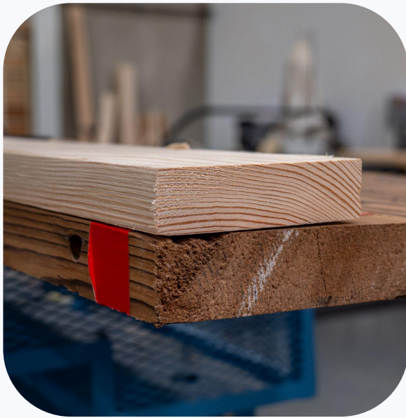
Squared and cleaned lumber next to the original salvaged condition of the wood.
