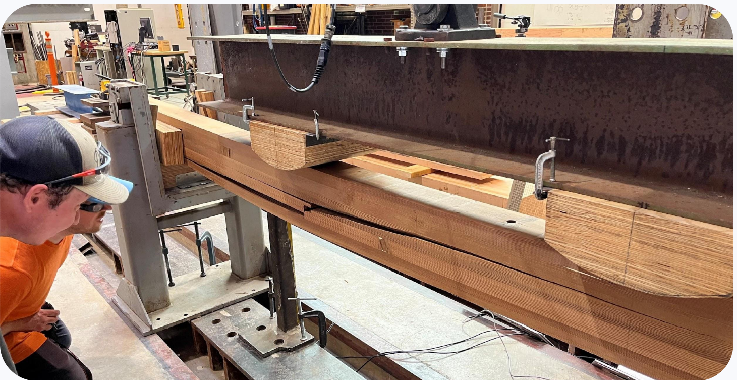
Wood strength and stiffness testing at Oregon State University's Wood Science and Engineering Lab.
