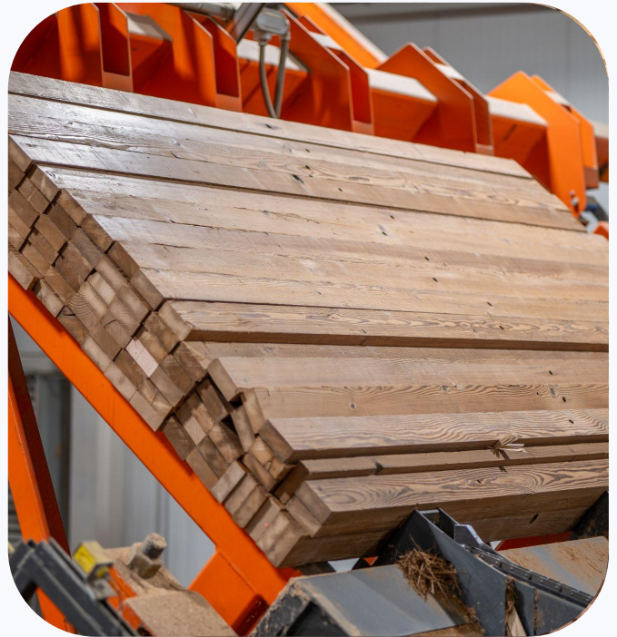
Cleaned and squared wood loaded for regrading.
