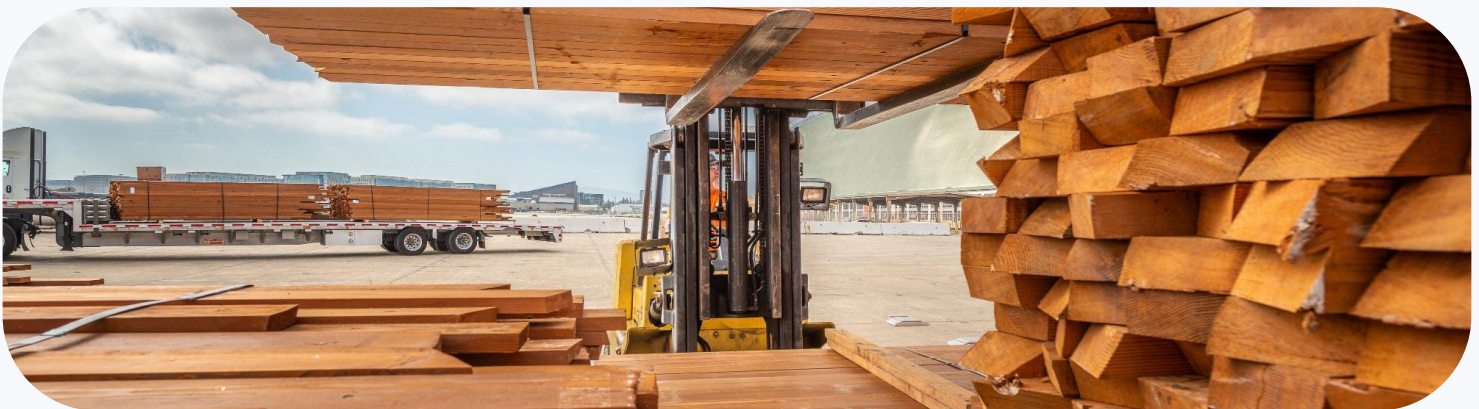
Salvaged boards are neatly stacked prior to loading to be shipped for testing and reuse.
